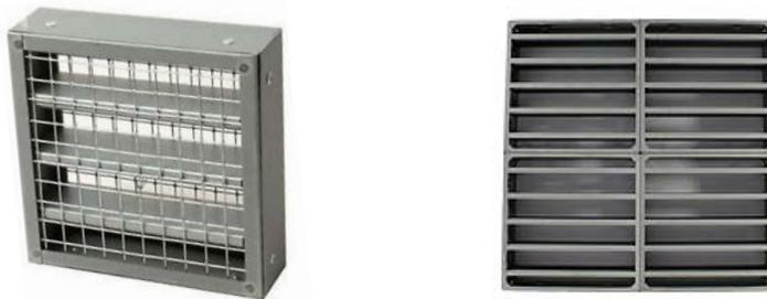
An intumescent vent permanently closes in the event of a fire. When overheated, a special material inside the vent expands greatly to block air flow and to prevent the spread of smoke and fire.
