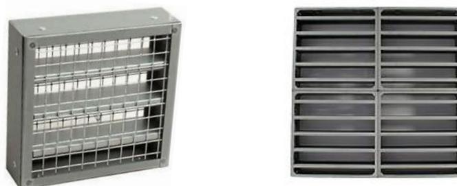
Intumescent vents are needed when ventilation must pass through a fire-resistant wall. They close when overheated in the event of a fire. A special material inside the vent expands greatly to completely block air flow. This limits the spread of smoke and poisonous gases and stops the vent from acting as a source of oxygen for the fire.
