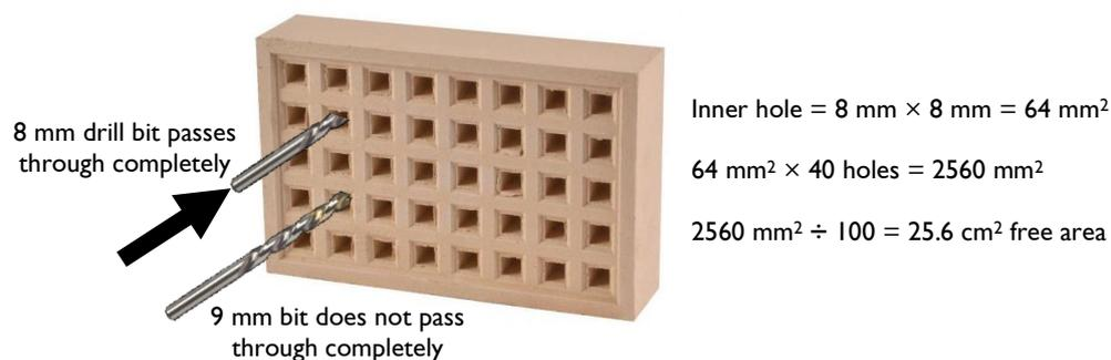
Air bricks are an acceptable form of air vent for gas appliances although their free area is small. They are often used in a supplementary role with other types of vent, or when ventilation requirements are just above adventitious allowance (page 8).
