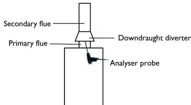
For the above appliance, if undiluted CO and CO<sub>2</sub> values in the primary flue are 200 ppm and 8 % (80000 ppm) respectively, the CO/CO<sub>2</sub> ratio will be  $200 \div 80000 = 0.0025$
