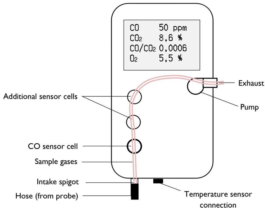
All combustion analysers have a CO sensor cell which allows them to measure the concentration of CO in appliance exhaust gases or in ambient air.
